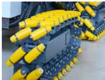
The drum-shaped rolls are mounted in an angle to the caterpillar track drive
